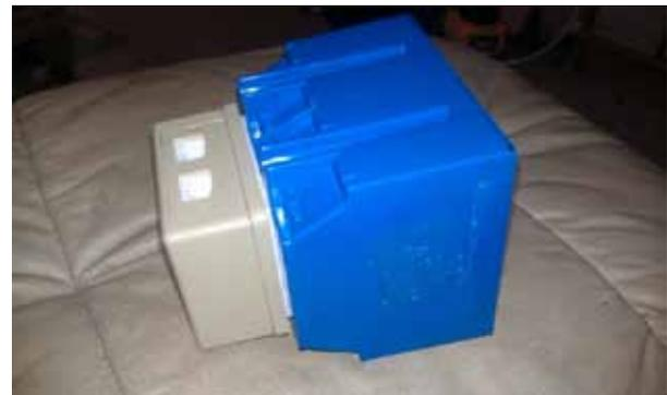
Trace the face onto some sort of 1/4" wood to be used as the mounting point for the UP5. This is used to cut out the opening for the UP5 and for the pilot holes for all the screws.
