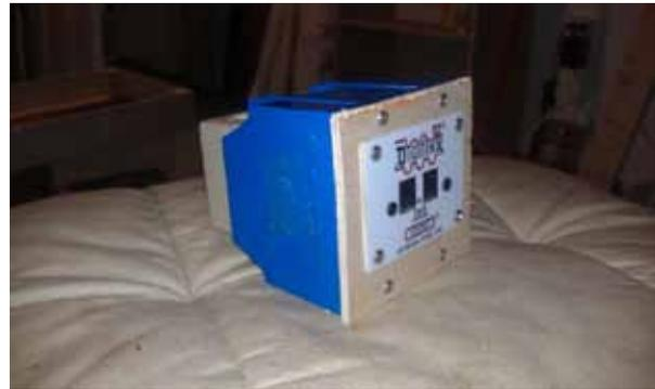
Mount the UP5 to the wooden face plate using 4 screws. Connect the two Loconet cables to the back of the UP5. Mount the wooden faceplate to the gang box using 4 screws.
