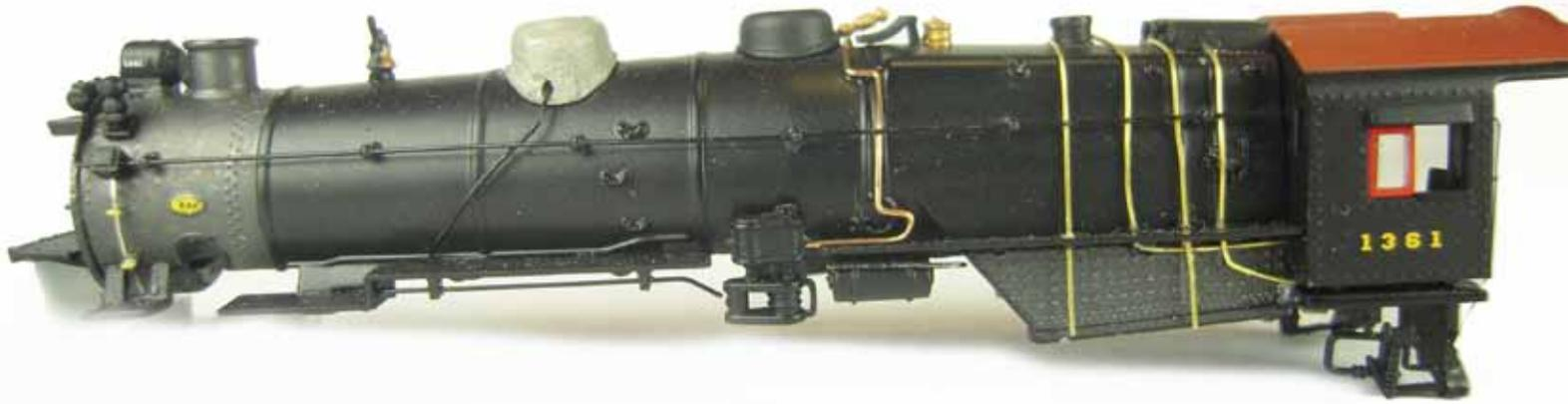
Photo 2: Cab roof painting and boiler piping
