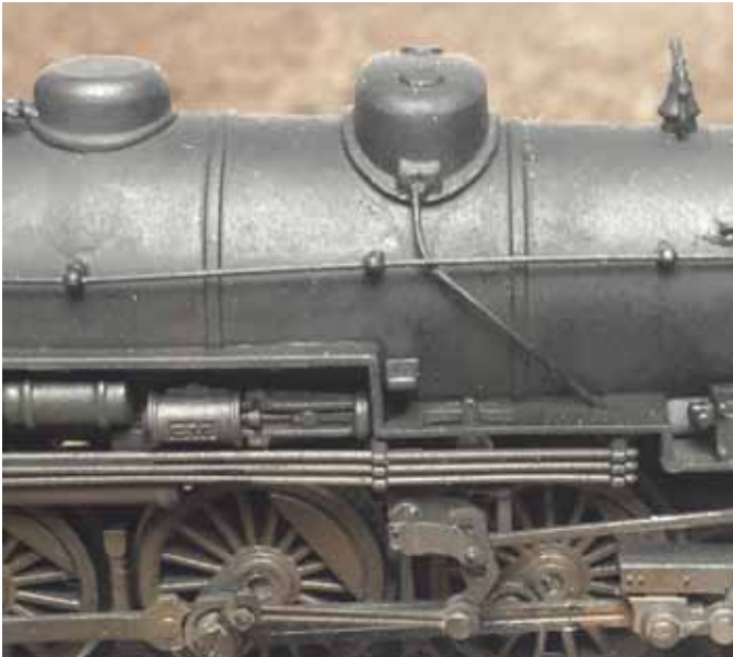
Photo 7: Weathering and Neolube highlights on boiler
