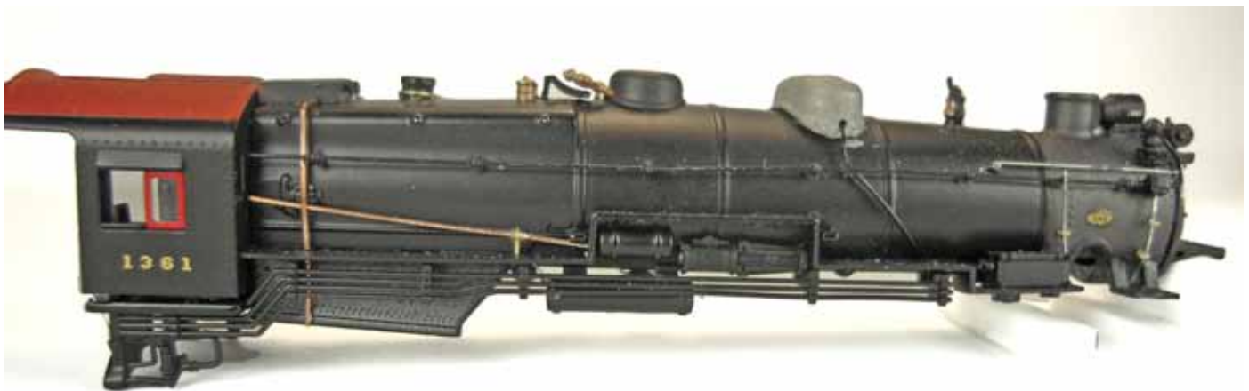
Photo 3: Right side piping with original cast metal replacement sand dome
