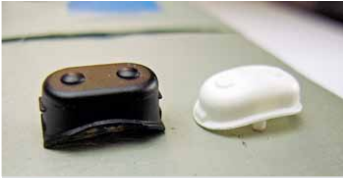
Photo 4: Original Bachmann sand dome (left) vs. replacement provided by John LeMerise
