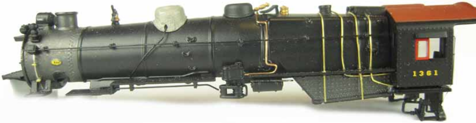
Photo 2: Cab roof painting and boiler piping
