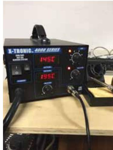
The unit is able to make the temperature changes quickly because the heating element is not a metal core as you find in most other irons. The heating element is a ceramic rod inclusive of a heating element, temperature sensor and ground surrounded by a metal tube, which attaches to a changeable tip. The changeable tip fits over the ceramic core.
