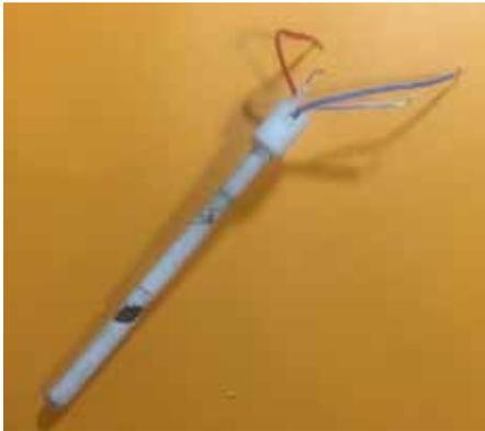
The significant downside of the machine is the Iron-heating element is a solder in unit. Think about that
