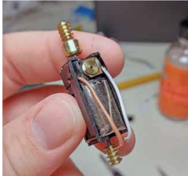
The removed motor in its cradle. Something about the way the wires are arranged can cause a short.
