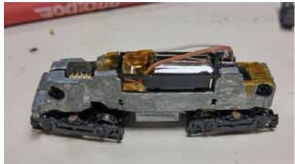
The solder pads on my decoders were too thick, so I had to give them a gentle, but firm, squeeze in some pliers to make them thin enough to fit into the slots in the mechanism. Finally, slide the decoder in and push the motor leads into the connectors.
