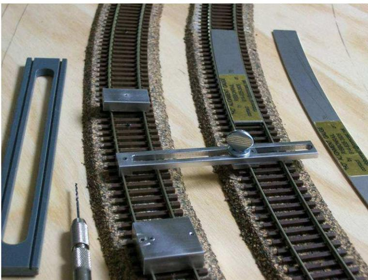
*Clockwise from left: MLR straight alignment tool, flex track drill jig, Ribbonrail curved track alignment gauges, adjustable curved/straight track parallel tool, power feed hole drill jig, pin vise with drill bit.*
