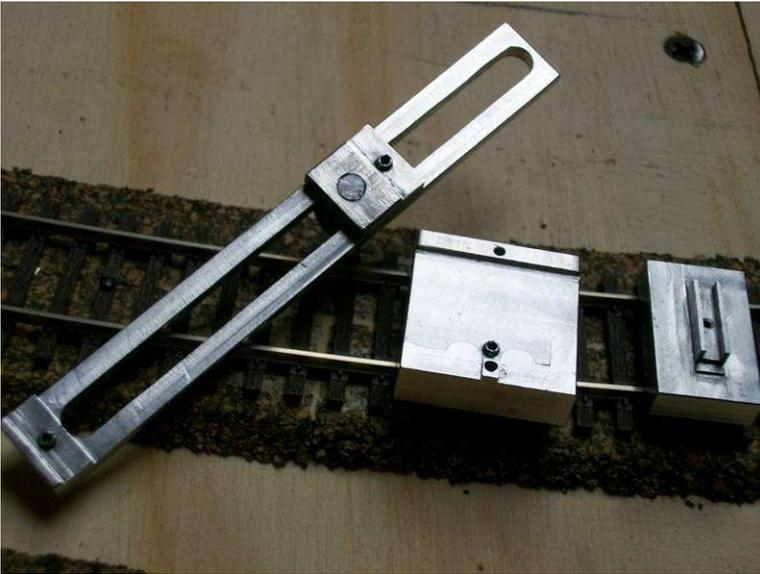
Left to right: adjustable curved/straight track parallel tool, power feed hole drill jig, flex track drill jig.
